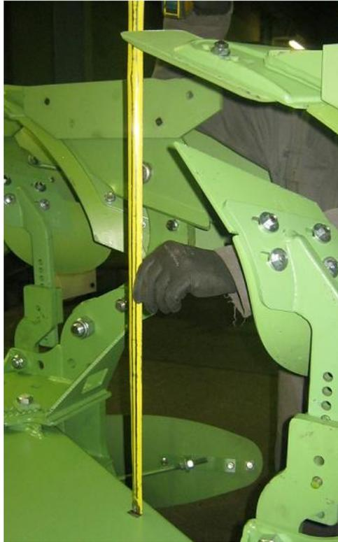
This should ideally be done with a new set of points as there may be different amounts of wear on a part worn set. On large ploughs it can be quicker to set the front and rear furrow then run a tensioned string from the front and rear furrow to set the bodies in between.
