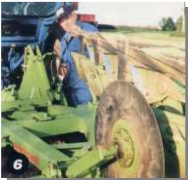
adjusted by slackening the two frog to leg bolts and the side hold bolt on the plate (for UCN/SCN only). The two adjustment bolts (or the eye bolt on YCN/DD bodies), can be used to move the required body in the correct direction (pic 7). When all bodies are the same level, run the string from the front point to the rear, and adjust the latter as necessary.
