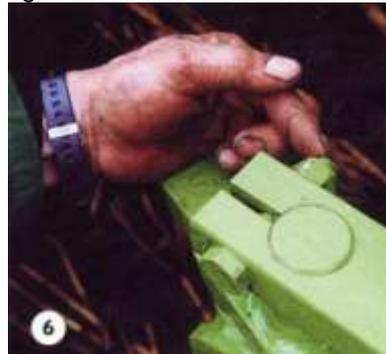
With regard to disc depth, the distance from the centre of the disc bearing hub to the point of the share should be set at least 7.5cm (3") greater than the maximum ploughing depth. To alter disc depth, remove the securing bolt (NB doubles also as a shearbolt), move the discs arm up or down as required and replace the bolt in an appropriate hole (pic 7).
