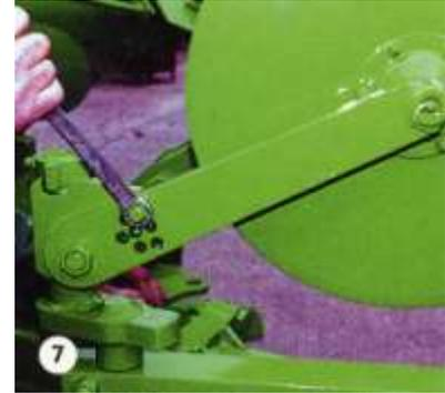
Final settings are best carried out in the field to suit the level of trash and the chosen ploughing depth. The disc should be set deep enough to cut through all surface trash and wide enough that it does not press hard against the skim in work.
