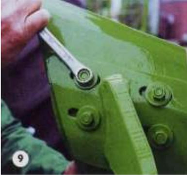
As with discs, final adjustment is best made in the field. The skim should be set deep enough to ensure that all stubble is deposited in the furrow bottom as the furrow is being turned. Lateral skim settings depend on trash levels. Higher levels of trash normally require skims to be moved closer to the land.
