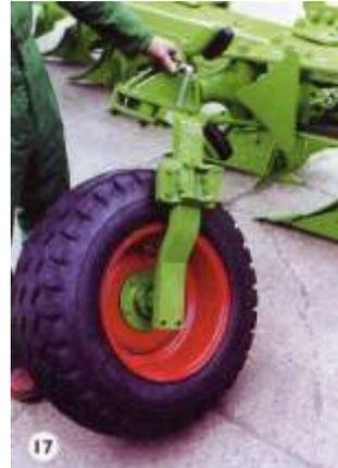
Moving to the front nearside of the plough, remove the lynch pin from left-hand transport locking pin, move the locking pin rearward and replace the lynch pin.
