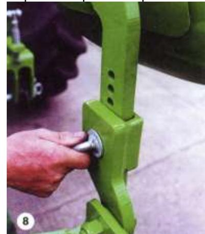
With regard to width, start by positioning the point of the skim approximately 1.9cm (3/4") outside of the share. Adjustment is made by slackening the four fastenings (pic 9) and sliding the skim
