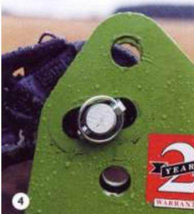
If the tractor has top link draught sensing, the top link should be positioned in one of the three circular holes in the ploughs headstock.
