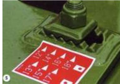
Note: The required furrow width is achieved when the centre of the appropriate arrow is in line with the centre of the bolt (shown at 14"). Rotate the serrated notch plate through 180 degrees to achieve odd or even width settings. The furrow width of HA models can be adjusted hydraulically from the tractors seat across the full width range.
