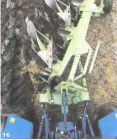
point can be moved if you find that the ram has reached the end of its stroke before the front furrow width has been set correctly, the aim must be to get the ram piston close to its central position in work.
