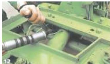
The latter should be greased before and after turning over the plough. Examine hydraulic hoses, check tyre pressures and replace any badly worn or broken parts.
