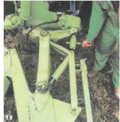
**120 MA;** Both alignment and offset may need to be altered to suit ploughing width and tractor wheel settings. Set the front furrow width adjuster ram to its mid position, then turn the offset adjuster handle (Fig 14) until the top link runs true. Finally, fine tune the front furrow width on the adjuster ram.
