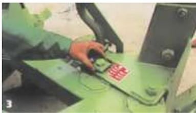
The centre of the arrow showing the widths must be in line with the centre of the bolt. Turning the washer through 180deg alters the setting between odd and even widths. Each leg and body can then be pivoted to the required position and the bolts retightened. 100 HA models are adjusted hydraulically in work.
