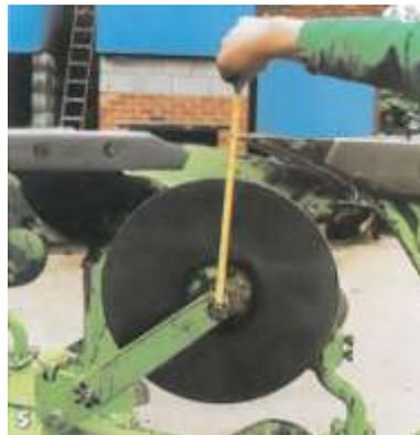
Adjust using multi-hole fixings in disc arm (fig 6).
