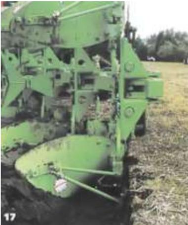
Adjust lateral attitude on vertical setting bolts. Fore and aft adjustment is made on the top link and the depth wheel. It is important that the plough sits level in work. Sloping forward will result in inadequate furrow turnover. Sloping rearward will result in poor penetration.
