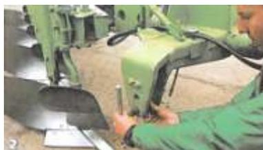
Under most circumstances, the tractor's lift arms should be connected to the lowest attachment holes on the plough (Fig 2). When ploughing deep, it may be necessary to use the upper holes to achieve the required depth.
