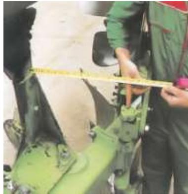
Adjust using bolt in slot securing disc bracket. To minimise wear and trash build-up, disc depth should be set so that the distance from the centre of the disc hub to the share point is at least 3in (75mm) more than maximum ploughing depth (fig 5).
