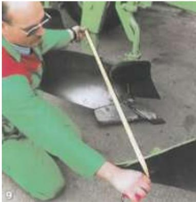
Check this distance on the opposite handed body. The measurements should be the same. Now, measure from the marks made on the centre bodies to the marks made on the remaining bodies. These should be the same as the interbody clearances specified for your plough. Adjustment is made by lengthening or shortening the mouldboard stay.
