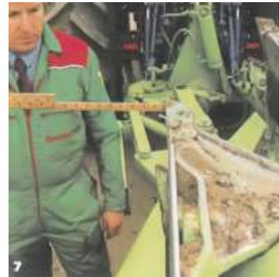
On 100 MA and 120 MA models, the rear disc should be set parallel, approximately 3/8in (9.5mm) wider than the landslide. The skim should be adjusted close to the disc, almost, but not quite touching.
