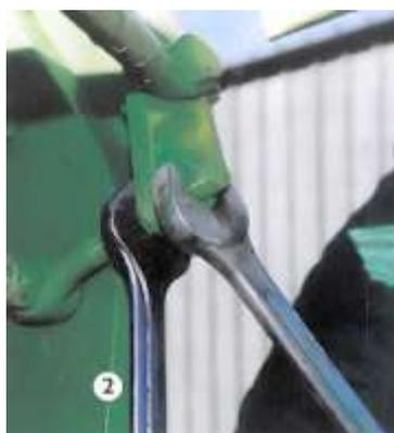
N.B Dowdeswell auto-reset ploughs still have shearbolts. One is fitted to each leg to provide secondary protection in case the point becomes jammed beneath an immovable object such as a tree root or bedrock, preventing the leg from swinging back. Two shearbolts are available (Pic 3), red for normal
