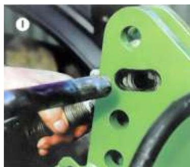
When using an auto-reset plough, It is recommended that the top link is fitted to the elongated hole in the ploughs headstock (Pic 1), enabling the plough to move independently of the tractor in work. This is
