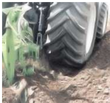
With no furrow wall to guide the wheels, a tractor running in a widened furrow bottom must be steered so that the outside of the front and rear wheels follow the edge of the final furrow turned on the previous pass.
