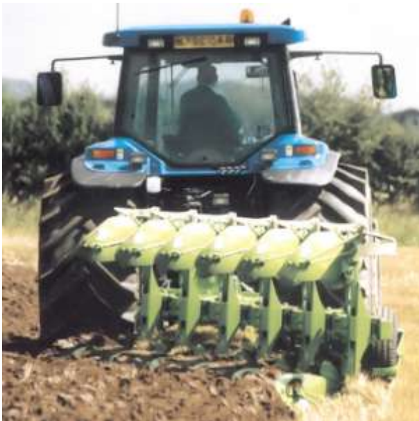
To plough successfully in the furrow with wide tyres, the tractor's wheels need to run in an enlarged furrow bottom produced by a furrow widener fitted to the plough's rearmost body.
