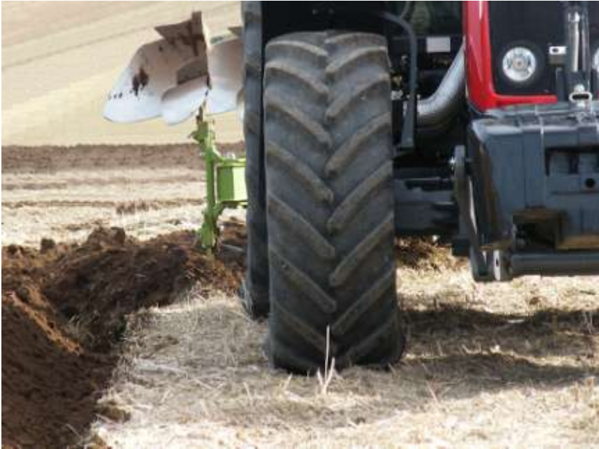
Ploughing on the land with a purpose designed plough. The additional offset built into the plough enable the tractor's over sized tyres to run one furrow width away from the work. Accurate steering is vital.
