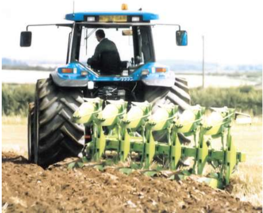
Ploughing an even and consistent furrow with oversized wheels on the tractor. The furrow widener which will come into work on the return pass can be seen fitted to the rear most body of the plough.
