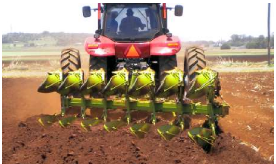
Working on-the-land with extra wide tyres keeps the tractor level and produces the widest possible footprint from the tyres. It is important that the tractors top link is kept in line with the direction of travel.
