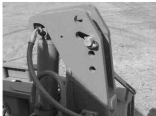
Where the tractor has lower link sensing, the top link pin should be located in the slot. When ploughing on level ground, the top link pin should be set to run in the centre of the slot, whereby allowing the pin to move forwards and backwards when ploughing over the undulations in the ground.
