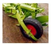
The auto-reset (FR) plough features a rear mounted pneumatic or steel depth wheel with independent left and right hand depth adjustment on a castoring bracket and hydraulic damper, for a smooth shock free turnover.
