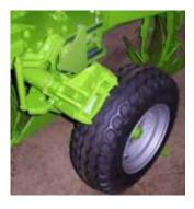
A combination depth / transport wheel can be fitted as a cost option on the shearbolt models. It has a spanerless depth adjustment and single pin movement from working position to transport position, allowing the plough to be transported in the 'butterfly' position.
