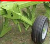
The shearbolt (FS) plough features a side mounted pneumatic or steel depth wheel with independent left and right hand depth adjustment and hydraulic damper, for a smooth shock free turnover.
